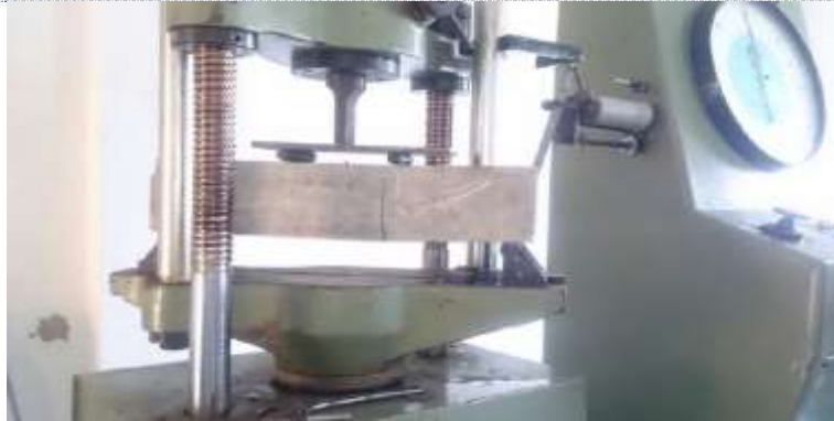
Fig. 2: Specimen loading for flexural strength test
